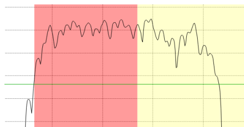
Figure 40: A signal breaking a flat baseline threshold and falling partially within an exclusion zone (the yellow shaded portion). Only the unexcluded part of the signal is considered an event (the red shaded portion).
