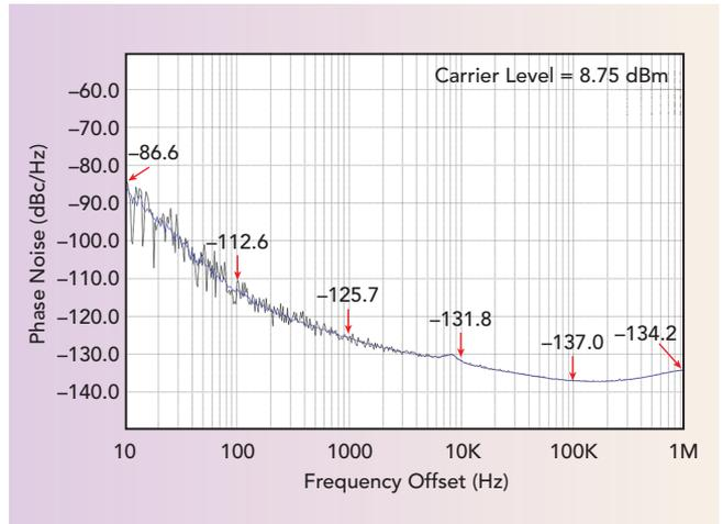
▲ Fig. 2 Measured phase noise of a 1 GHz reference signal from Signal Hound's phase noise clock standard.
