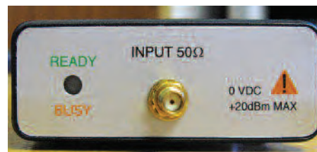
PHOTO 2: Front of SA44B analyser. The front of the TG44 tracking generator is similar.
